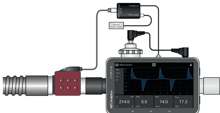
Figure 29: Placement of the MultiGasAnalyser
