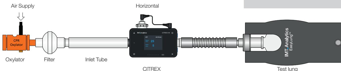
After presetting the CITREX flow analyser and arranging the correct set up, the Oxylator can be started.
