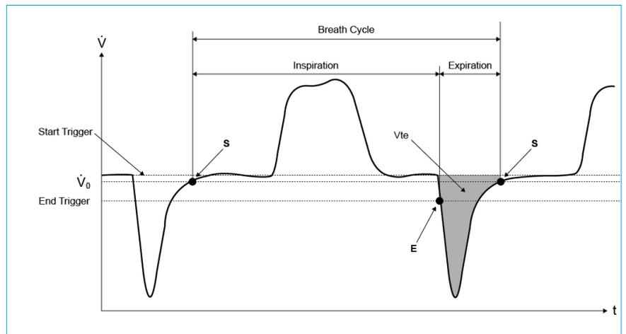
Here, the start trigger should be also placed at S and the end trigger should be placed at E.
