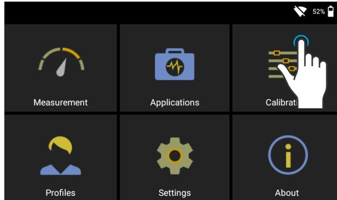
In the Calibration sub-menu tap the **Zero Offset** icon. Follow the instructions on the screen and tap **Start**. After successful calibration a confirmation appears. The device is now ready for use.
