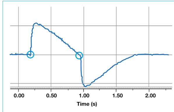
This example shows a flow curve downstream of the Y-piece. The standard triggers (> 3 L/min / < -3 L/min) can be used in this case without any problems.
