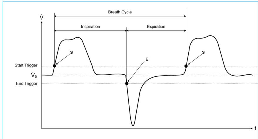
Correct definition of the start and stop triggers is therefore of major importance and it can have a considerable impact on the measurement results.
