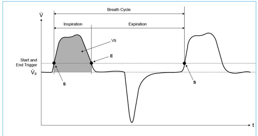
S on this chart represents the start trigger and E represents the end trigger.
